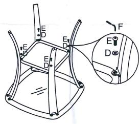
STEP 2: Assemble table tray (C) to 4 table legs (A) by using 4 screws (E) and 4 washers (D) with allen wrench (F). Do not tighten all bolts now.
